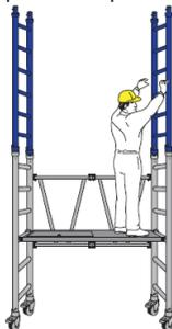
2. Erect the diagonal braces. Clip diagonal braces onto the lowest rung of the second set six rung ladder frames, clip the other ends onto the opposite frame rung. Ensure to lock them entirely.
