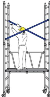
3. Locate the adjustable stabilisers. Fix the upper end of the stabiliser onto the second set ladder frame, & lower end on to the first set ladder frame.
