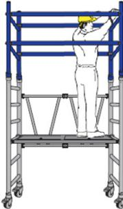
2. Move the platform with hatch to the top of the first set ladder frame.
